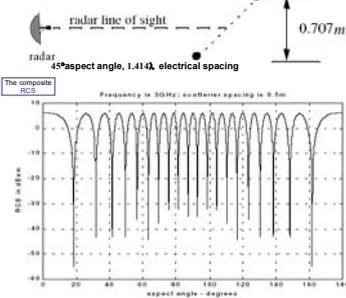
Knowledge of this constructive and destructive interference between the individual scatterers can be very critical when trying to extract RCS of complex or maneuvering targets. Reasons: 1) the aspect angle may be continuously changing; 2) complex target RCS can be made up from contributions of many individual scattering points distributed on the target surface (scattering centers).
